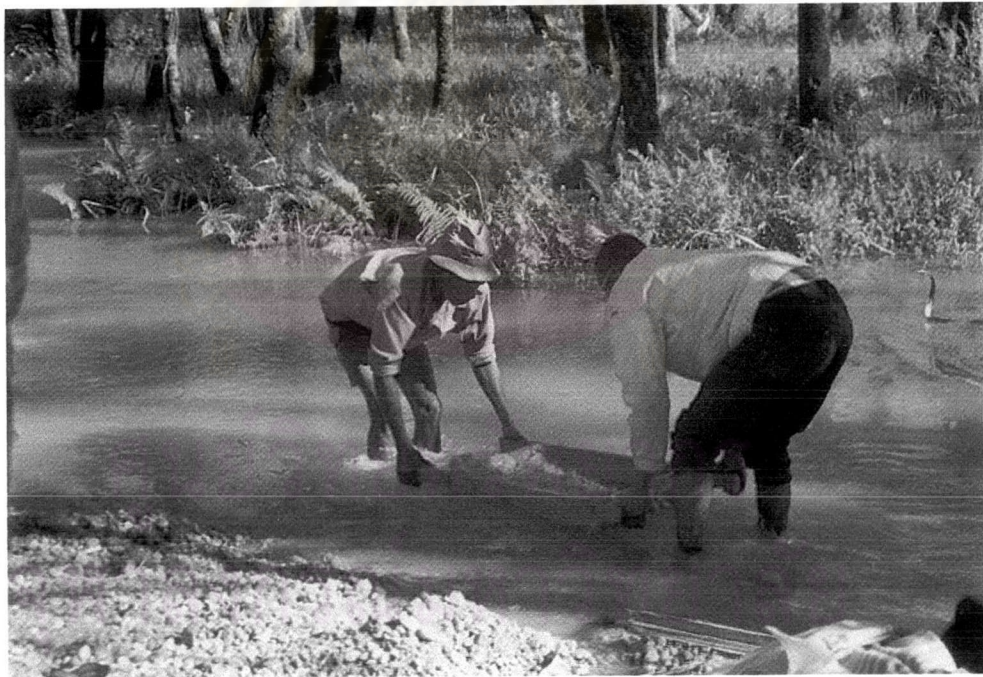
Figure 2.6 Panning and washing gravels along the Ilakaka river (Pezzotta et al., 1999)
