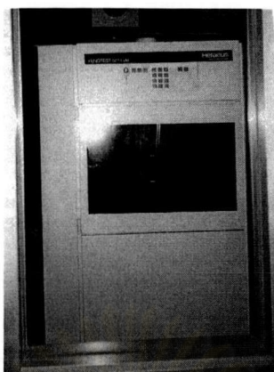
Figure 3.3 The Xenotest Beta Lamp chamber for accelerated UV
