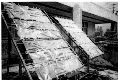
Figure 3.2 The exposure racks for outdoor exposure study
