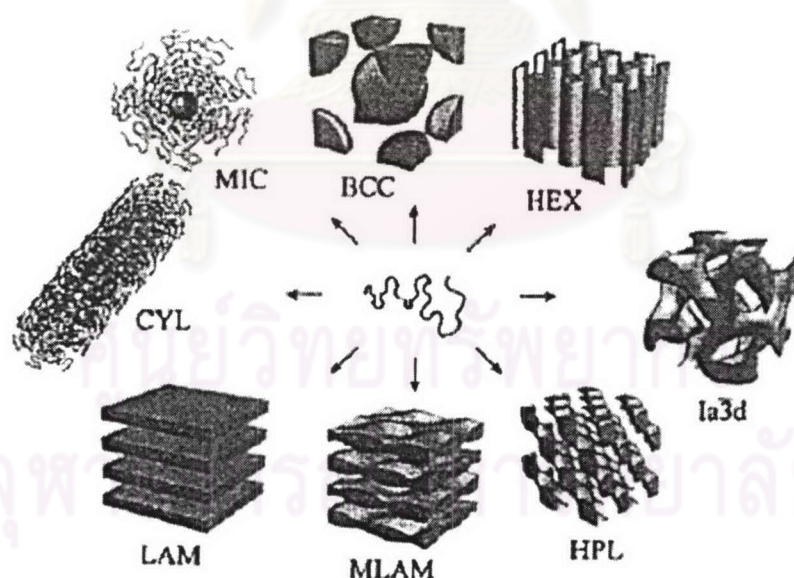
Figure 2.17 Main morphologies of block copolymer: spherical micelles (MIC), cylindrical micelles (CYL), lamellar structures (LAM), modulated lamellar (MLAM), hexagonal pinhole layers (HPL), gyroids ( Ia3d ), ordered cylinders (HEX), and body-centered cubic (BCC). 73
