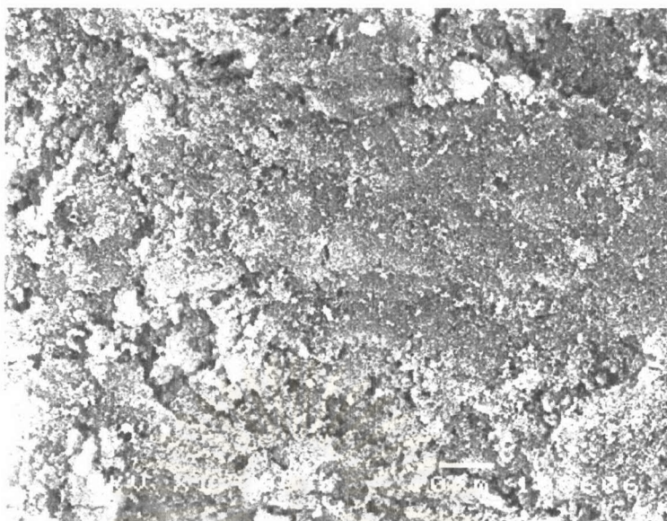
Figure 4.10 SEM photomicrograph of grafted PMMA
