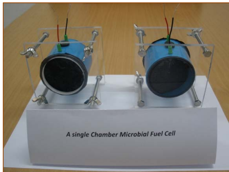
Figure 3.1: A single chamber microbial fuel cell used in the study
