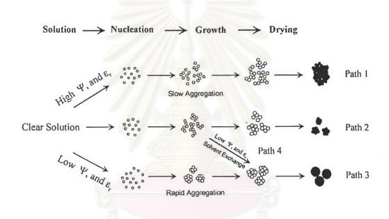
Figure 2.1 Schematics of particle growth in the mixed solvent of alcohol and water. (Park et al., 1997)
