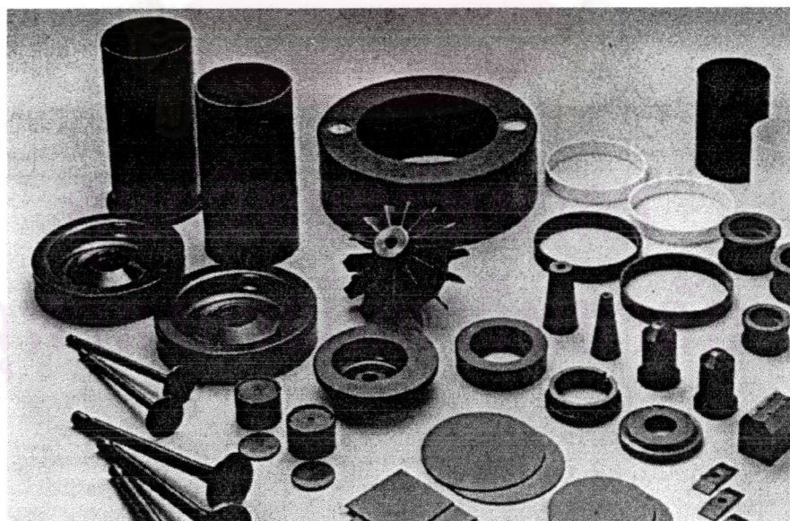
Fig 2.1 Silicon nitride components, including other materials (Partially stabilized zirconia (white) and aluminum substrates (thin plates)). 24)
