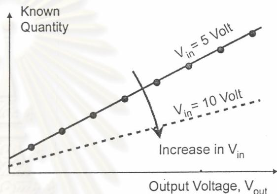
Normalization of Voltage giving Unique Slope called Calibration Factor, CF
