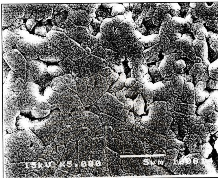
SEM micrograph of 0.5% MgO doped AKP-30 alumina sintered at 1600 °C 2 hours
