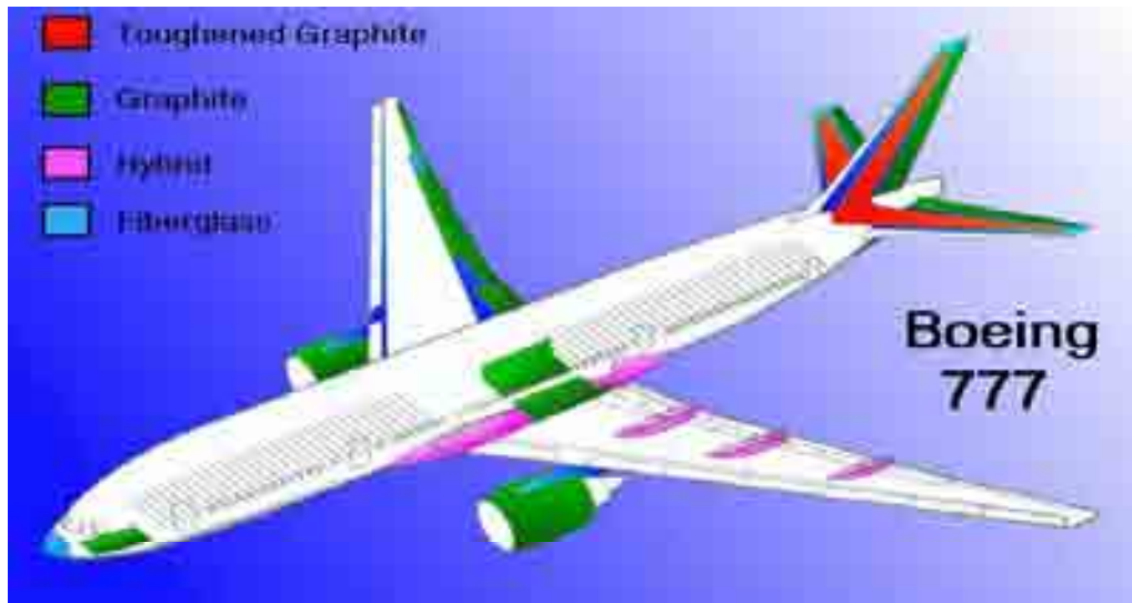
Figure 2.3 Various composite materials are used in structures of the Boeing 777 [24]
