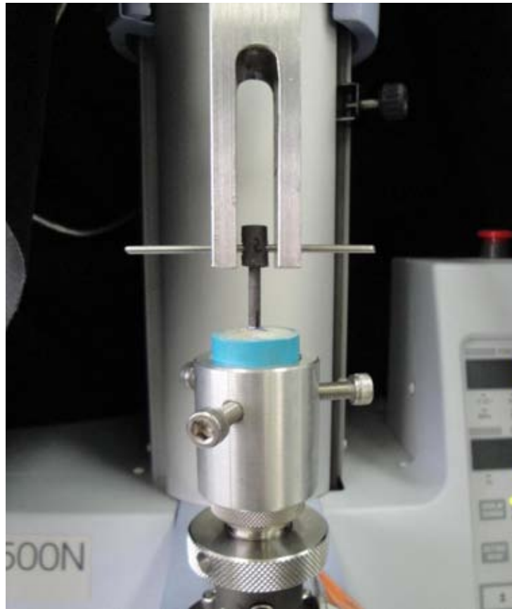
Figure 11. Specimen mounted to universal testing machine
