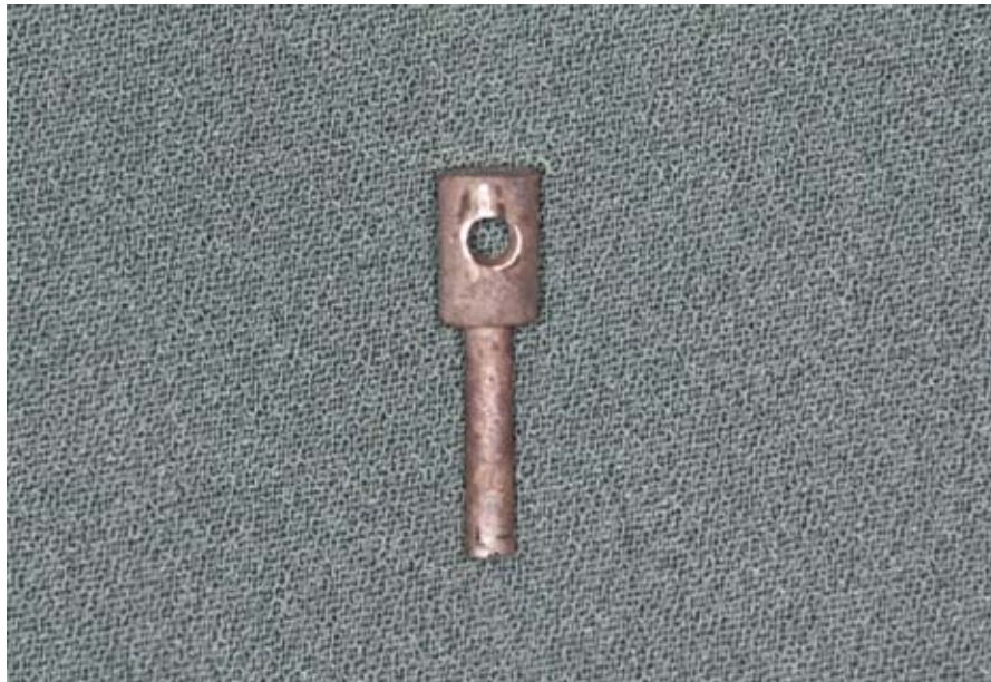
Figure 7. Metal specimen with 3-mm hole on setting up side
