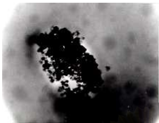
Figure 17 Transmission electron micrograph of capsule prepared by using \text{TiO}_2 as core material.
