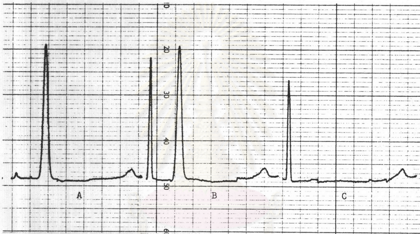
Figure 7. Chromatogram Fluorescence Intensity of A. Methyltestosterone B. Mixture of methyltestosterone and water-soluble vitamins C. Water-soluble vitamins
