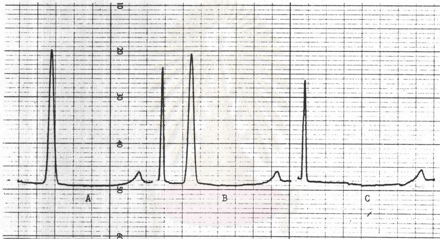
Figure 9. Chromatogram Fluorescence Intensity of A. Methyltestosterone B. Mixture of methyltestosterone and other compounds C. Other compounds
