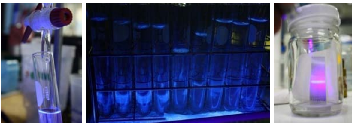
Figure 3.16 Fluorescence emission of 1,4-DHPs under black light lamp
