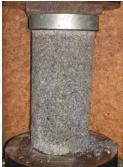
Figure 3.8 Compressive test on pervious concrete
