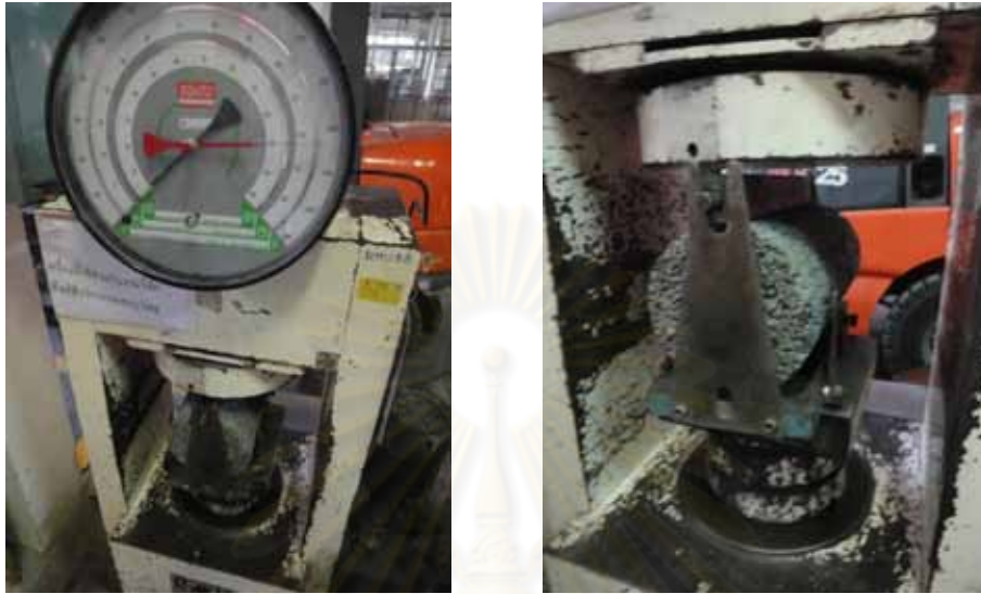
Figure 3.9 Splitting tensile strength test of pervious concrete
