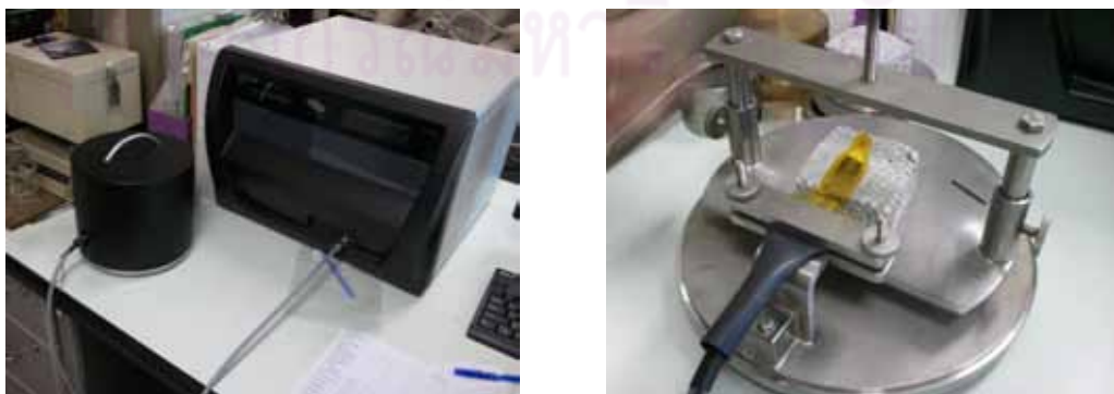
Figure 3.10 Apparatus for testing the thermal conductivity
