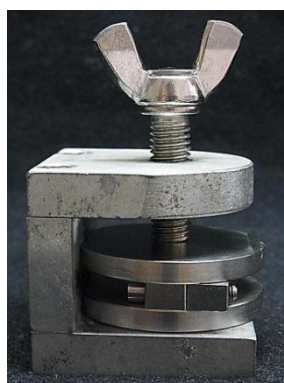
Figure 9 Clamp for Compressive Strength Test
