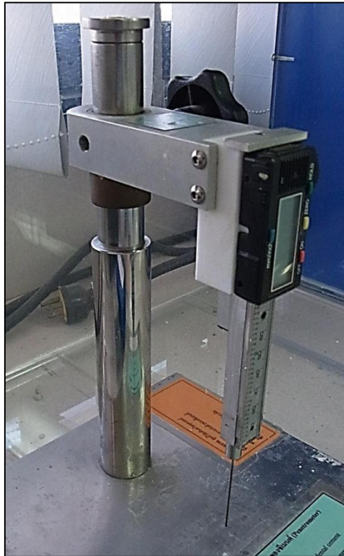
Figure 7 Indenter, 400\pm 5 g Flat End (Needle Size 1.0\pm 0.1 mm)
