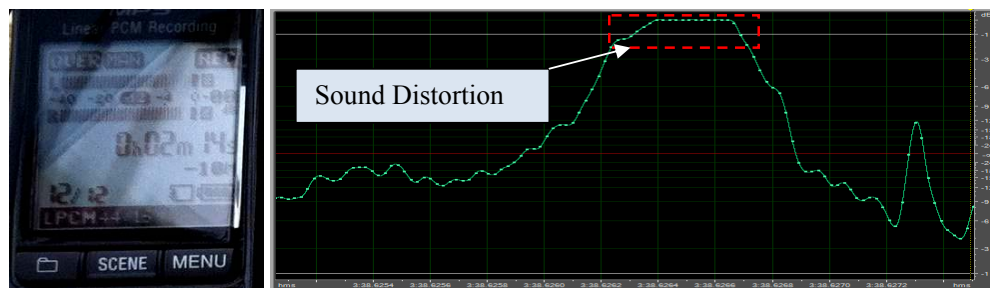
Figure 4.8 Sound distortion presented in sound signal
