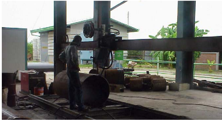
Figure 3.5 Longitudinal Welding Station
