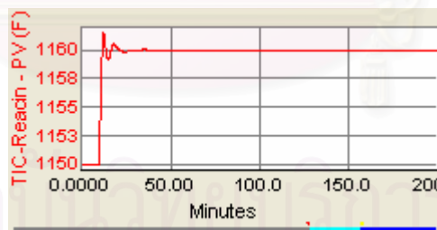
Figure 4.28a Dynamic response of increase 10 °F in reactor inlet temperature of CS6
