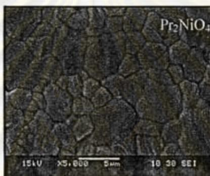
**Figure 3.10** Surface morphology of  $\text{Pr}_2\text{NiO}_4$  disc.
