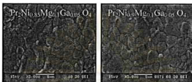
**Figure 3.20** Surface morphology of  $\text{Pr}_2\text{Ni}_{0.85}\text{Mg}_{0.1}\text{Ga}_{0.05}\text{O}_4$  and  $\text{Pr}_2\text{Ni}_{0.9}\text{Mg}_{0.1}\text{Ga}_{0.05}\text{O}_4$  discs.
