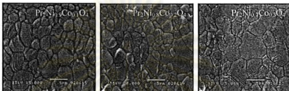
**Figure 3.13** Surface morphology of  $\text{Pr}_2\text{Ni}_{1-x}\text{Co}_x\text{O}_4$  ( $x = 0.1, 0.2, 0.3$ ) discs.
