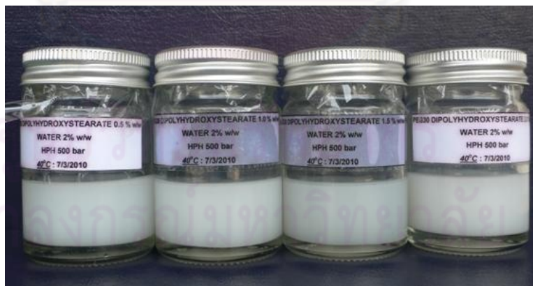
Fig. 16. Appearance of w/o nanoemulsions formulated with different emulsifier concentrations (0.5, 1, 1.5 and 2%w/w) after being kept at (a) 4°C, (b) 25°C and (c) 40°C for 3 months.
