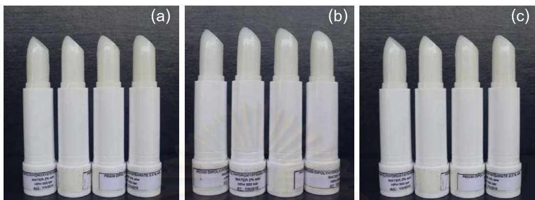
Fig. 21. Appearance of w/o nanoemulsion lipsticks formulated with different emulsifier concentrations (0.5, 1, 1.5 and 2%w/w) after 3-month storage at (a) 4°C, (b) 25°C and (c) 40°C.
