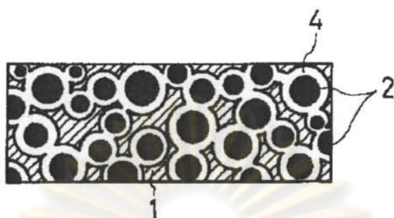
Figure 4.29 The sectional view after removing a surfactant, as it becomes the path 4 of the solvent [10].
