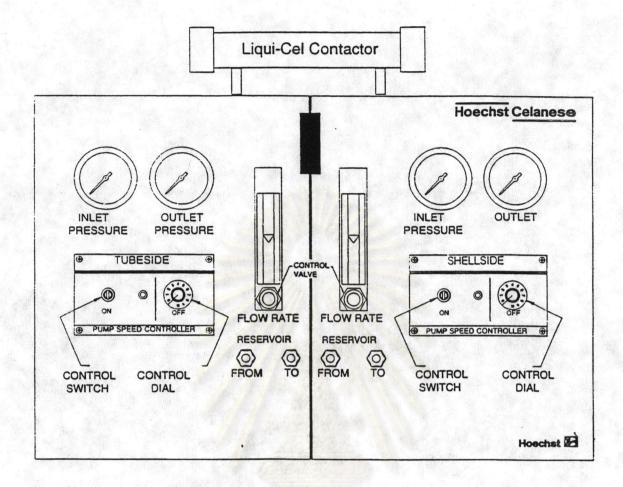
Figure 3-1 The Liqui-Cel Laboratory Liquid/Liquid Extraction System equipped with the Liqui-Cel Membrane Contactor
