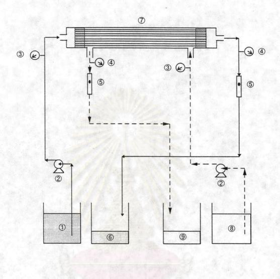
Figure 3-3 Schematic countercurrent-flow diagram for once-through-mode operation in HFSLM experiments where ① the feed solution reservoir, ② gear pumps, ③ inlet pressure gauges, ④ outlet pressure gauges, ⑤ flow meters, ⑥ the raffinate reservoir, ⑦ the HFSLM contactor, ⑧ the strip solution reservoir, and ⑨ the concentrated solution reservoir
