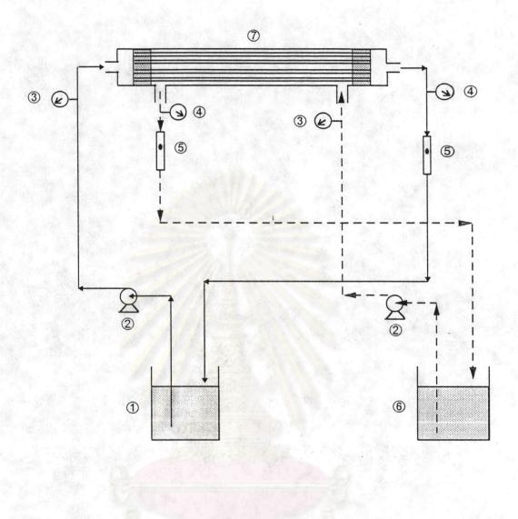
Figure 3-2 Schematic countercurrent-flow diagram for circulating-mode operation in HFSLM experiments where ① the feed reservoir, ② gear pumps. ③ inlet pressure gauges, ④ outlet pressure gauges, ⑤ flow meters, ⑥ the strip reservoir, and ⑦ the HFSLM contactor
