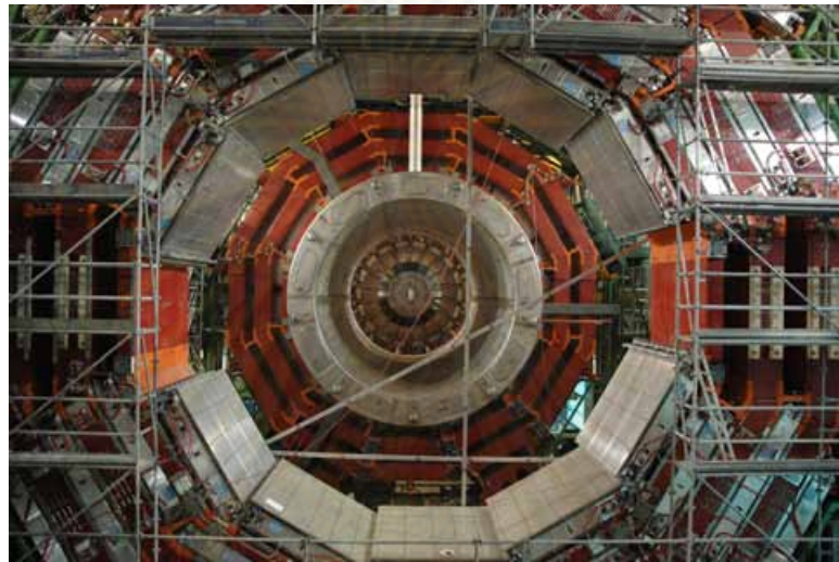
Figure 3.14: The complete CMS magnet coil (central part of picture) and the magnet return yoke (red part around center).
