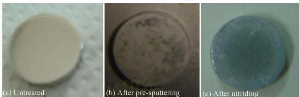
Figure 4.1: Surface morphology of a) Untreated sample, b) After pre-sputtering with Ar-H 2 for 1 h, and c) After nitriding with N 2 - H 2 for 25 h
