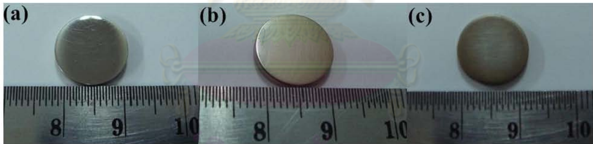
Figure 5.1: The comparison of surface color after nitriding of: (a) 1h, (b) 9 h, (c) 12 h.
