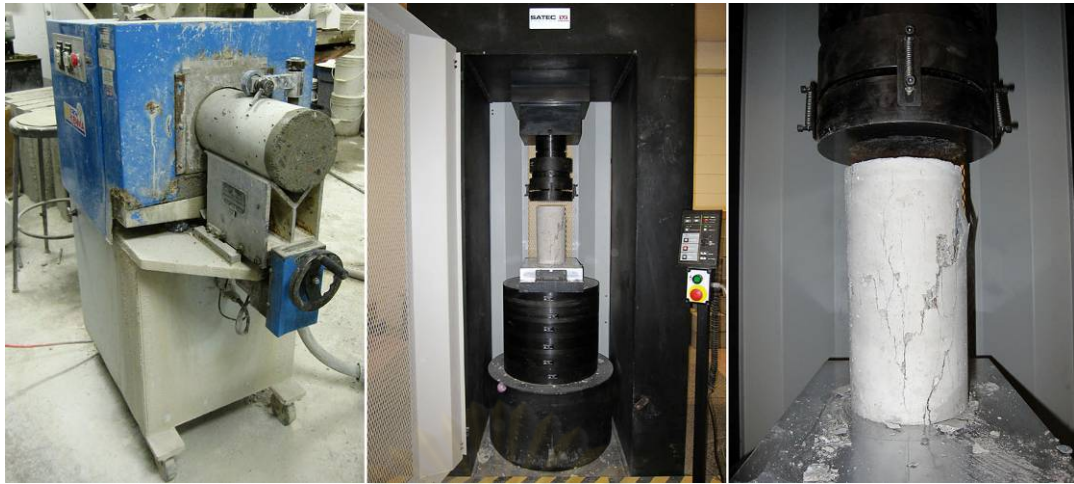
Figure 3.13 Concrete compressive strength tests
