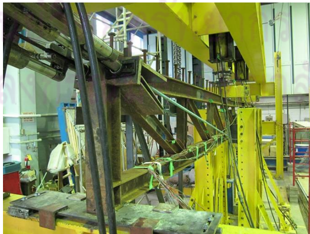
Figure 3.31 Specimen B2 – Lateral buckling at the ultimate stage.
