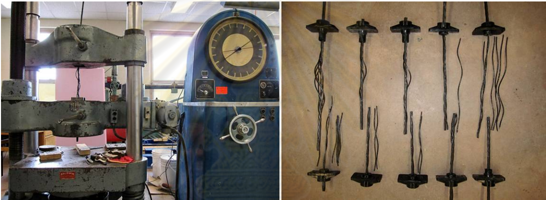
Figure 3.16 Monostrand unbonded tendon tension tests
