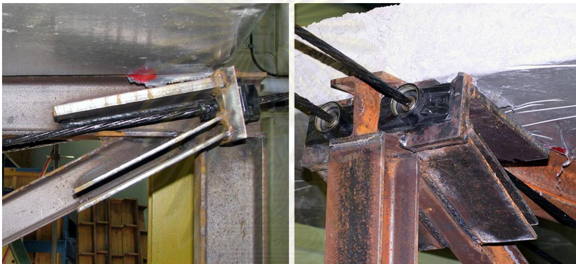
Figure 3.7 End anchorages of prestress tendons
