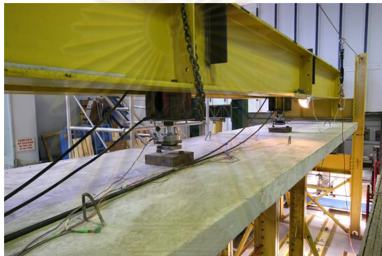
Figure 3.9 Two 1000kN load-rams with the load cells.
