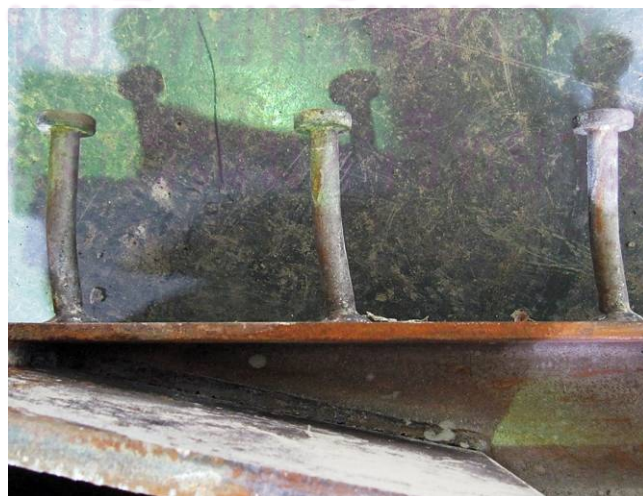
Figure 3.26 Shear stud connectors - inelastic deformed shape.
