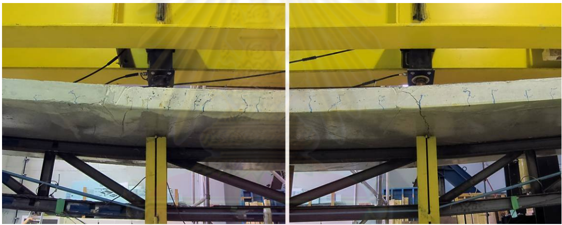
Figure 3.25 Cracks in concrete slab - Specimen A3.
