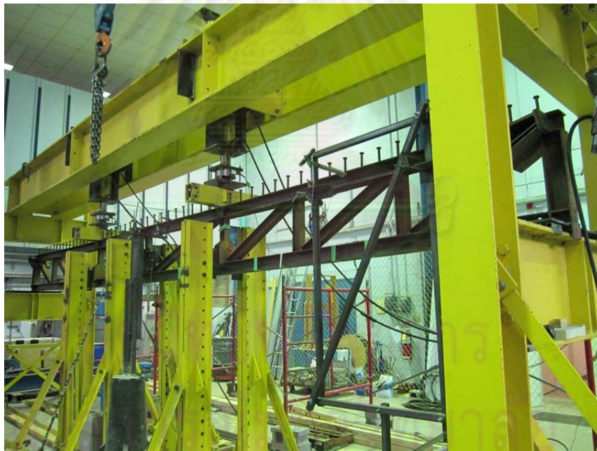
Figure 3.28: Specimen B1 - Steel truss only without tendon.
