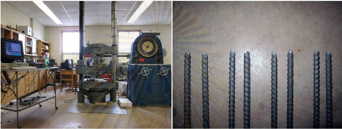
Figure 3.18 Tension tests of the slab rebar.
