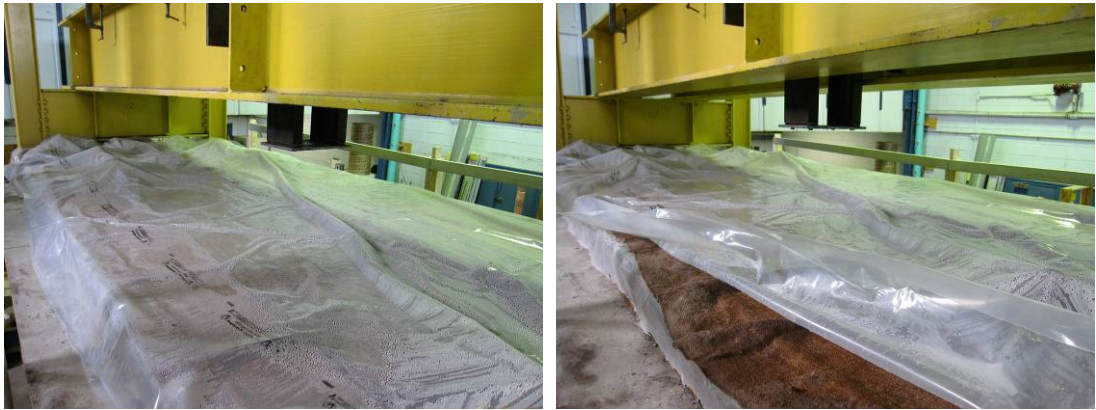
Figure 3.5 Curing under cover of wet burlap and plastic sheet.
