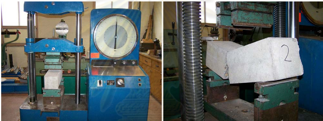
Figure 3.14 Concrete modulus of rupture tests
