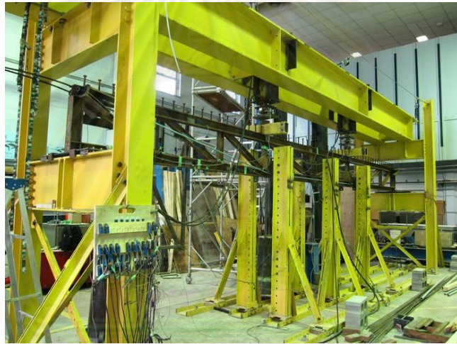
Figure 3.30 Specimen B2 - Steel truss with posttensioned tendons.
