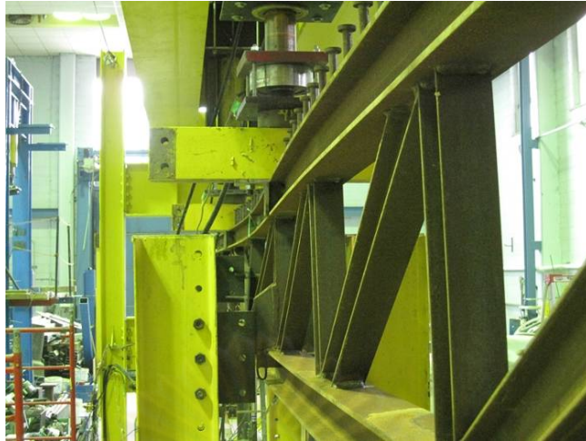
Figure 3.29: Specimen B1 - Lateral buckling of compression chord.
