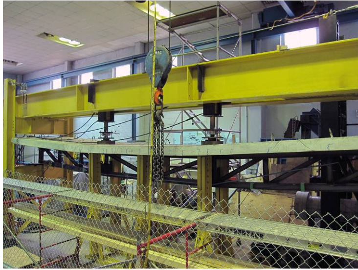
Figure 3.24 Truss series A showing Specimen A3 at ultimate.
