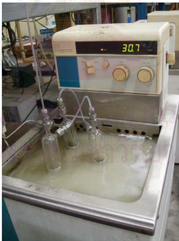
Figure C.3 Saturators for preparation of BTEX vapor.
