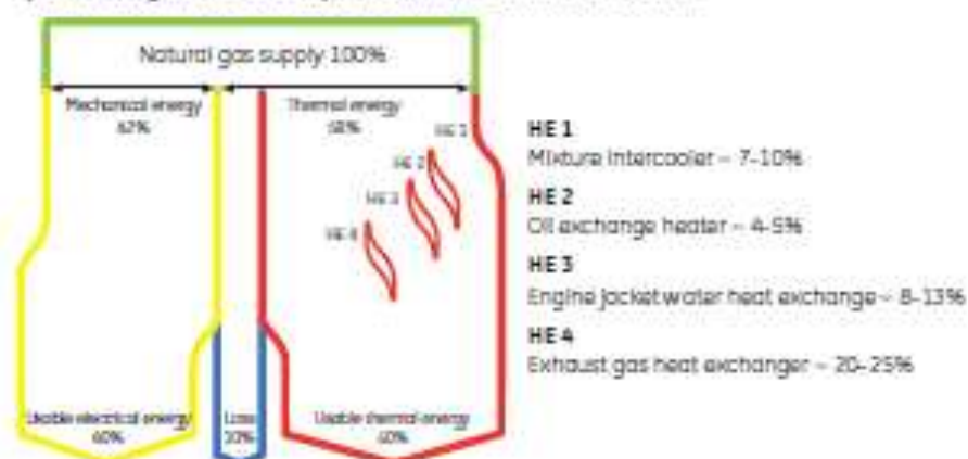
Figure 10. Sankey diagram of typical CHP application with typical gas reciprocating engine
