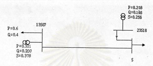
From one-line diagram as above. The load of transformers SD13507 and SD23518 (rated 500 kVA) were 378 kVA and 256 kVA respectively. The load could be increased by about 366 kVA. So in the simulation will the load increase be as follows:
