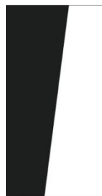
Figure 2.8 Slanted edge selected from ISO 12233 chart
