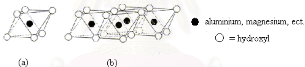
Figure 2.2 (a) A single octahedral unit (b) sheet structure of octahedral unit arranged in a hexagonal network.
