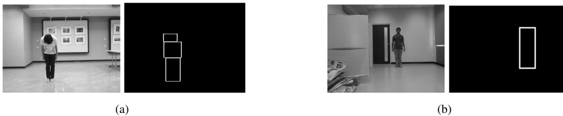
Figure 3.14: An example of bending and standing in a far distance postures with their corresponding posture envelopes. (a) Bending in 90^\circ viewing angle in near distance and its posture envelope. (b) Standing in far distance and its posture envelope.
