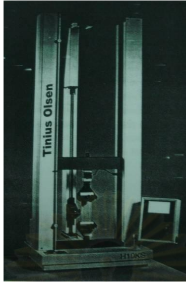
Figure 2.7 A universal testing machine used to measure tensile properties.
