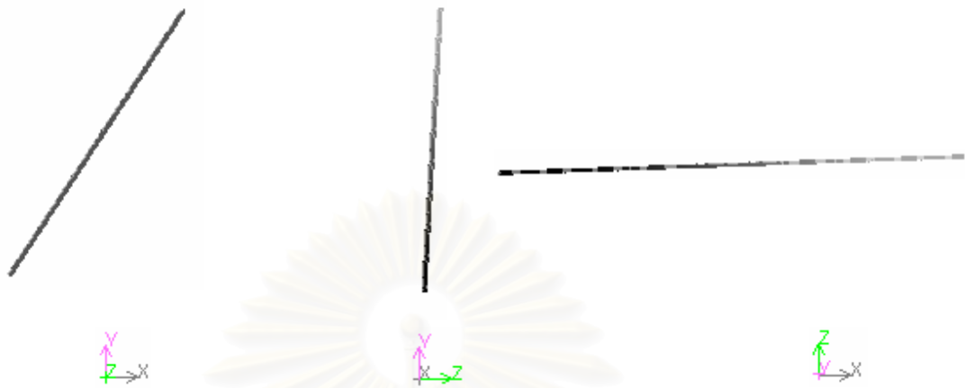
Figure 4.6 The conformation of single chain PE, 500 repeating units at 0 K.
