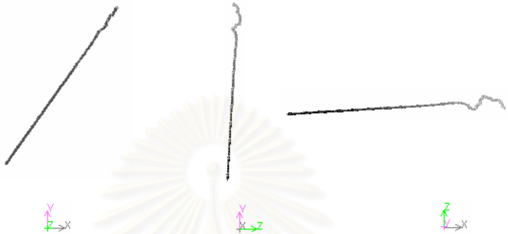
Figure 4.24 The conformation of single chain EPM, 500 repeating units at 0K.
