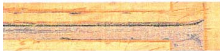
Figure 3.5 Snapshot of parallel flows that have smooth interface in microchannel (Zhao et al., 2006)
