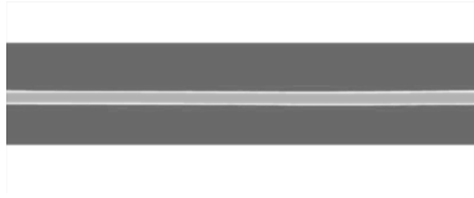
Figure 4.2 2D simulated stable stratified flow of the air (dark gray) and water (light gray) at superficial velocities of 20 and 0.4 m/s, respectively
