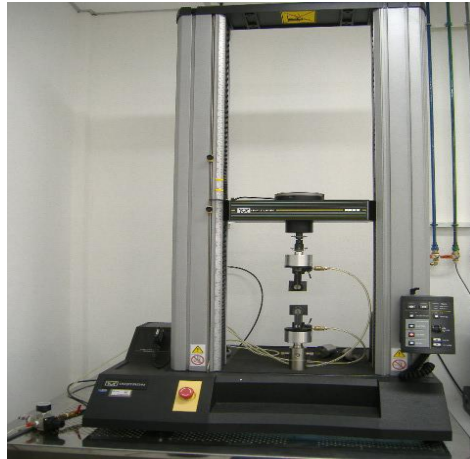
Figure 4.12 Tensile testing machine equipment [104-105].
