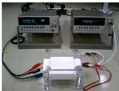
Figure 4.11 Current generator and Nanovoltmeter equipped with Four-point probe (Platinum wires) [104-105].
