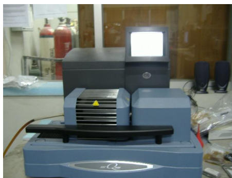
Figure 4.9 Thermogravimetric analysis (TGA) Equipment [104-105].
