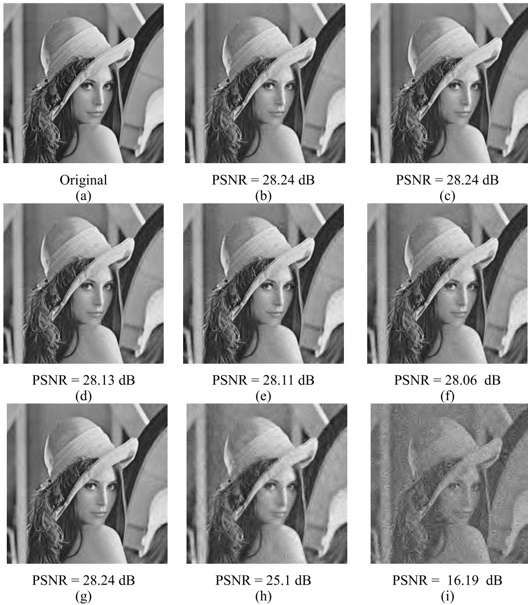
Figure 4.9: The reconstruction of Lena at M/N = 0.40 , \mu = 7y_{max} , p = 0.10 . (a) original image, the reconstructed images by (b) GBF at g = 1\% , (c) GBF at g = 2\% , (d) GBF at g = 5\% and (e) GBF at g = 10\% , (f) GBF at g = 20\% , (g) AMP, (h) HUBER, and (i) LIHT.
