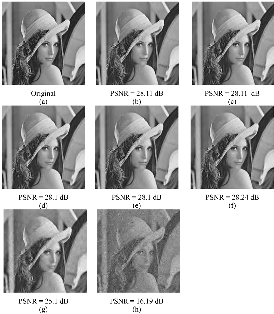
Figure 4.19: The reconstruction of Lena at M/N=0.40 , \mu = 7y_{max} , p = 0.10 . (a) original image, the reconstructed images by (b) GSSF at c = 0.125 , (c) GSSF at c = 0.25 , (d) GSSF at c = 0.5 , and (e) GSSF at c = 1 , (f) AMP, (g) HUBER and (i) LIHT.
