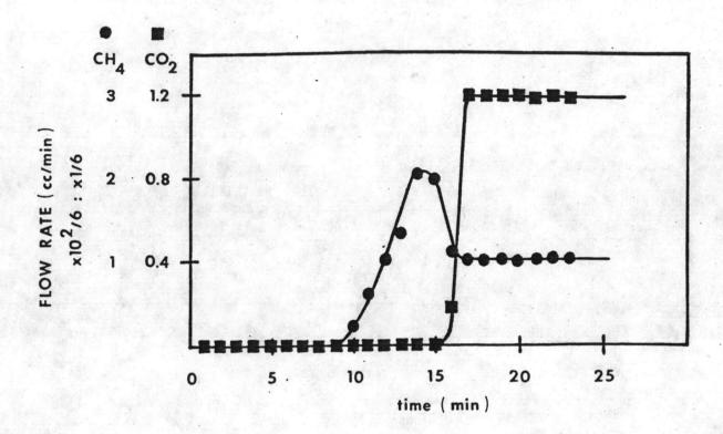
Figure 3.3 The breakthrough curve of mixture of carbondioxide and methane at 0.5 bar and 45 °C.
