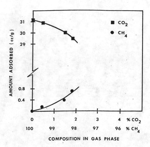
Figure 3.4 The equilibrium curve of a mixture of methane and carbondioxide at 45 °C and 0.5 bar.
