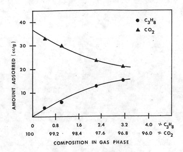
Figure 3.5 The equilibrium curve of a mixture of carbondioxide and propane at 45 °C and 0.5 bar.
