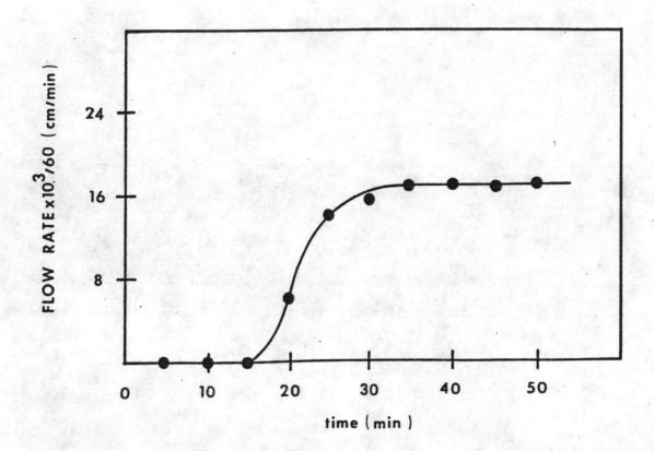
Figure 3.2 Breakthrough curve of carbondioxide at a partial pressure of 0.0685 and at 45 °C.
