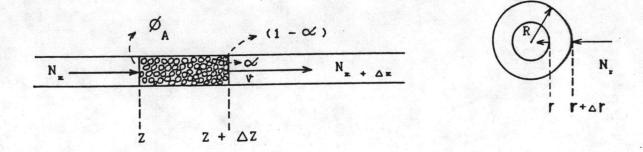
Figure 3.1 Component balance in gas phase and in particles.
