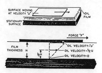
Figure 2-1: Concept of dynamic viscosity
