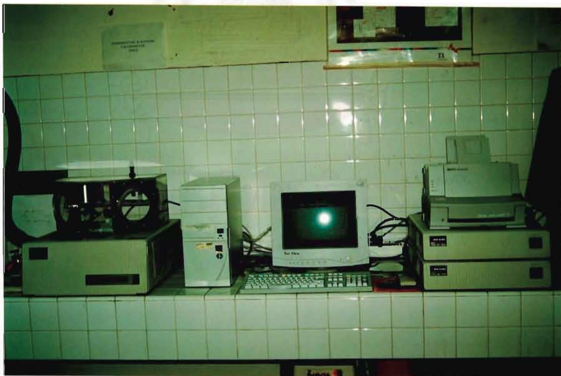
Figure 3.4 Differential Scanning Calorimeter (DSC7)
