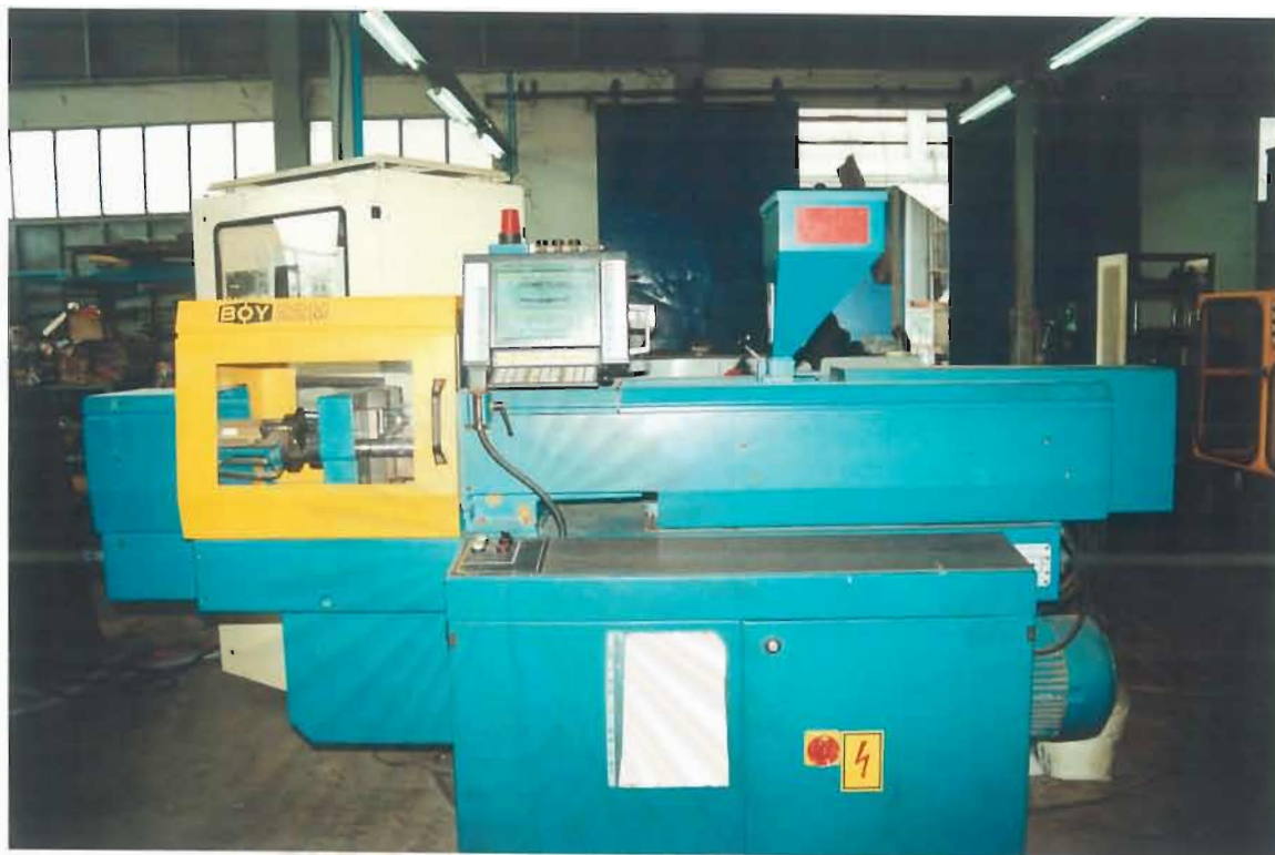
Figure 3.1 Injection Molding Machine.
