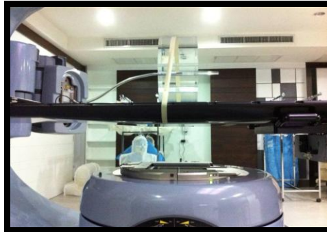
Figure 3.14 The chamber and phantom setting up on Exact IGRT couch
