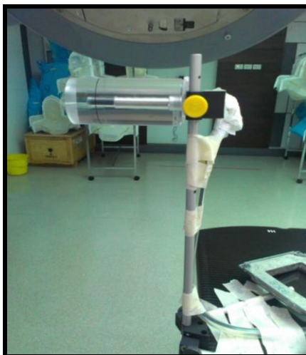
Figure 3.11 The chamber with buildup setting up on Varian Clinac iX linear accelerator
