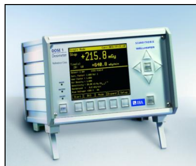
Figure 3.6 The DOSE-1 dosimeter
