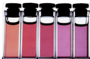
Figure 2.4 The color of colloidal gold nanoparticles in a varied solvent refractive index. Refractive indices of the solutions (from left to right) are 1.336, 1.407, 1.481, 1.525 and 1.583 [49].
