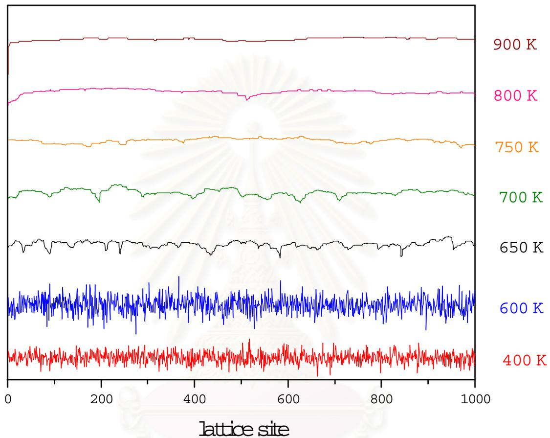
Figure 3.1: The surface morphologies of the MBE model for  $T = 400$  K, 600 K, 650 K, 700 K, 750 K, 800 K, and 900 K after depositing  $10^3$  ML on a substrate of size  $L = 10^3$  lattice sites. For low substrate temperature  $T = 400$  K and 600 K, the surface is very rough. For higher temperature, the surface morphologies become smoother.
