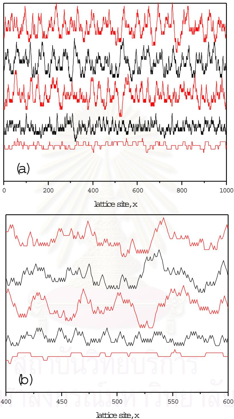
Figure 3.7: The surface morphologies of lattice mismatch model for  $T = 650$  K, substrate site = 1000 at 10 ML when strain energy increase. Strain energy = 0, 0.8, 1.2, 1.6, 2.0 eV from bottom to top. a) Show the morphology entire substrate and zoom in to show morphology of 200 lattice sites(400-600) in b).
