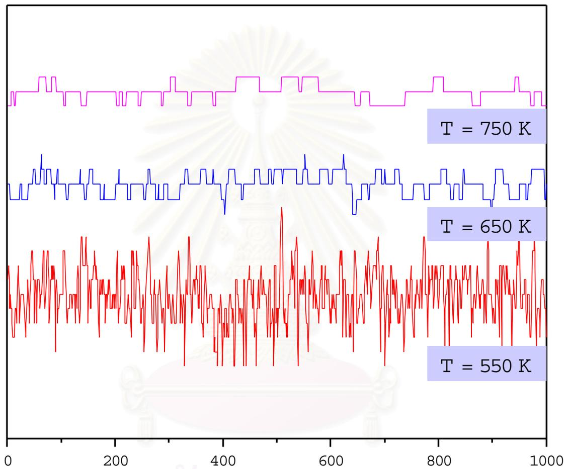
Figure 3.3: The surface morphologies of lattice mismatch model without strain for substrate temperature 550 K, 650 K and 750 K from bottom to top at 10 ML.
