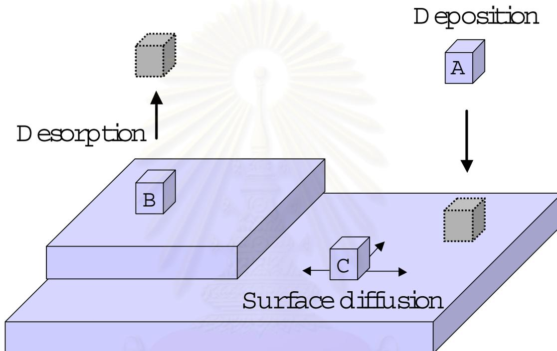
Figure 2.1: The MBE growth mechanism that taking place on the surface. (A) Atoms arrive on the surface, where they are deposited. (B) An atom on the surface may desorb, leaving the surface of the thin film. (C) Atoms diffuse in random directions on the surface.
