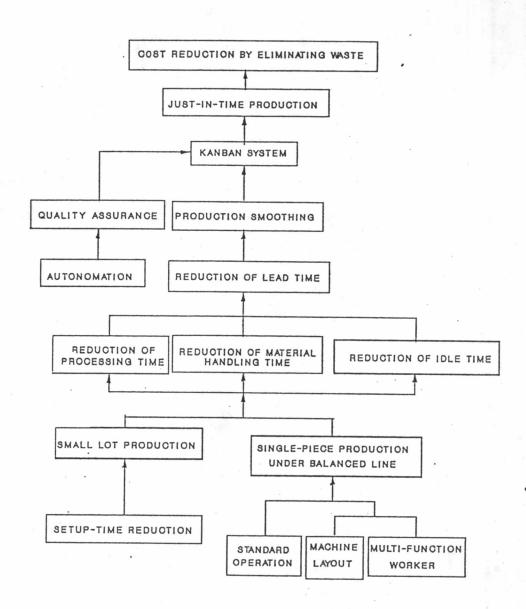
Figure 5.1. The way to reduces manufacturing lead time.
