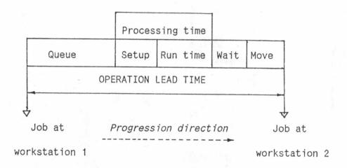
Figure 5.2. Operation lead time.
