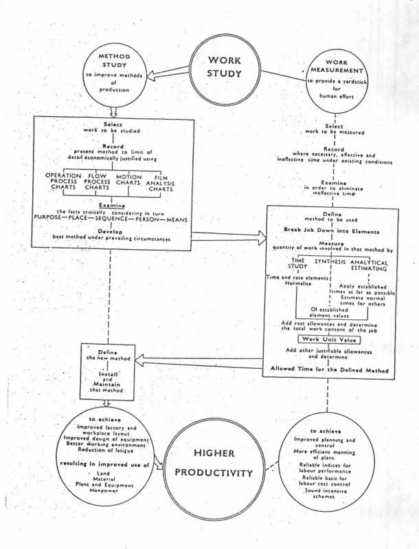
Figure 2.2. The inter-relation between method study and work measurement.
