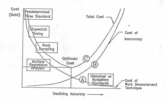
Figure 2.3. Cost vs. inaccuracy of work-measurement techniques.
