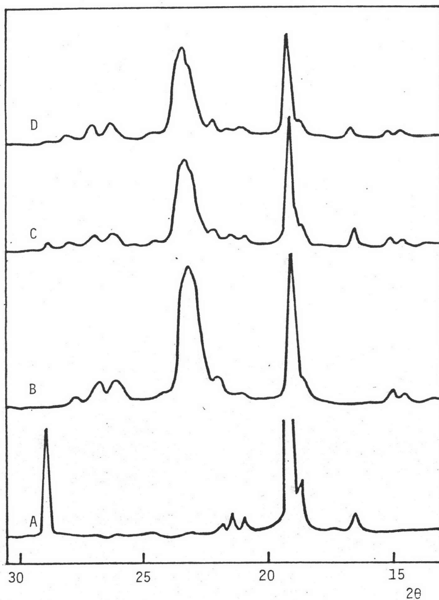
Figure 32 X-ray diffraction spectra of HCTZ-PEG 20000 systems Key: A, HCTZ alone; B, PEG 20000 alone; C, 1:10 HCTZ-PEG 20000 physical mixture; D, 1:10 HCTZ-PEG 20000 melt.
