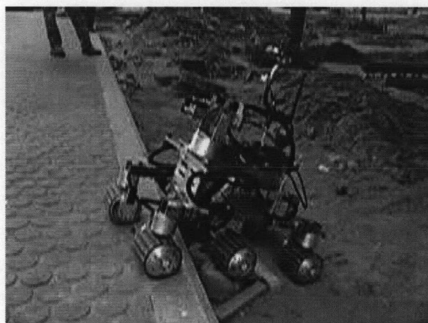
Figure 6.34: Climbing up the pavement.
