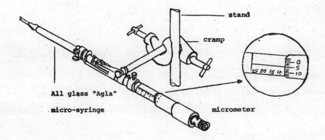
Fig. 4 All glass "Aglass" micro-syringe and micrometer
