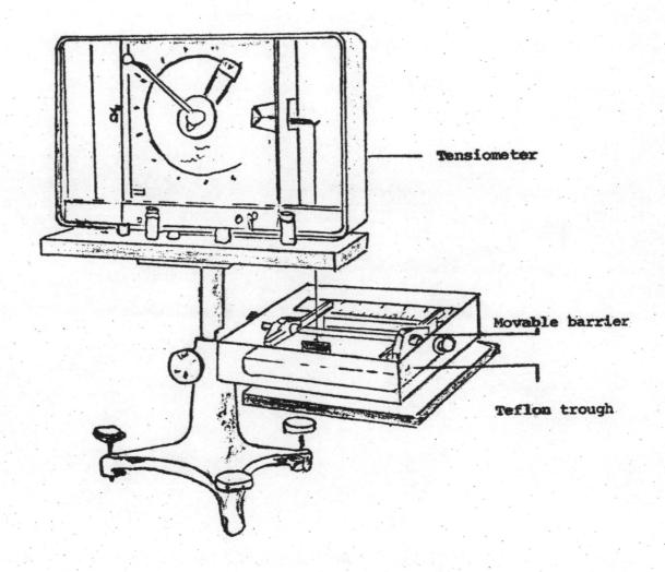
Fig. 5 Tensiometer with teflon trough and movable barrier
