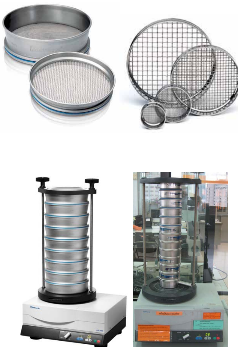
Figure 2.3 Sieve mesh and vibratory sieve shaker was used to select and collect comminuted peanuts (Available from: http://www.retsch.com/products/sieving/sieve-shakers/as-200-digit )
