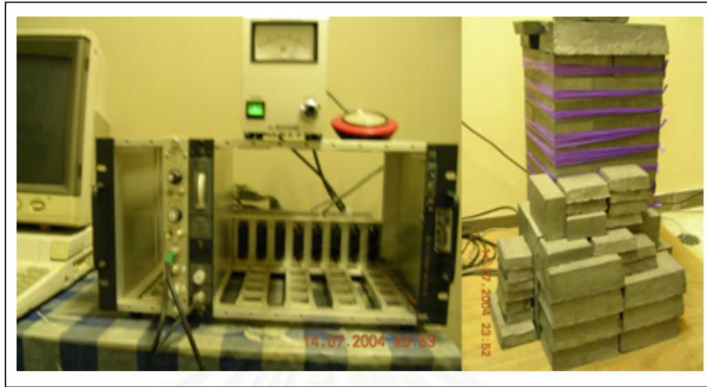
Figure 2.22 Gamma ray spectrometer at Akita University, Japan. This equipment is used for measure uranium, thorium and potassium contents.
