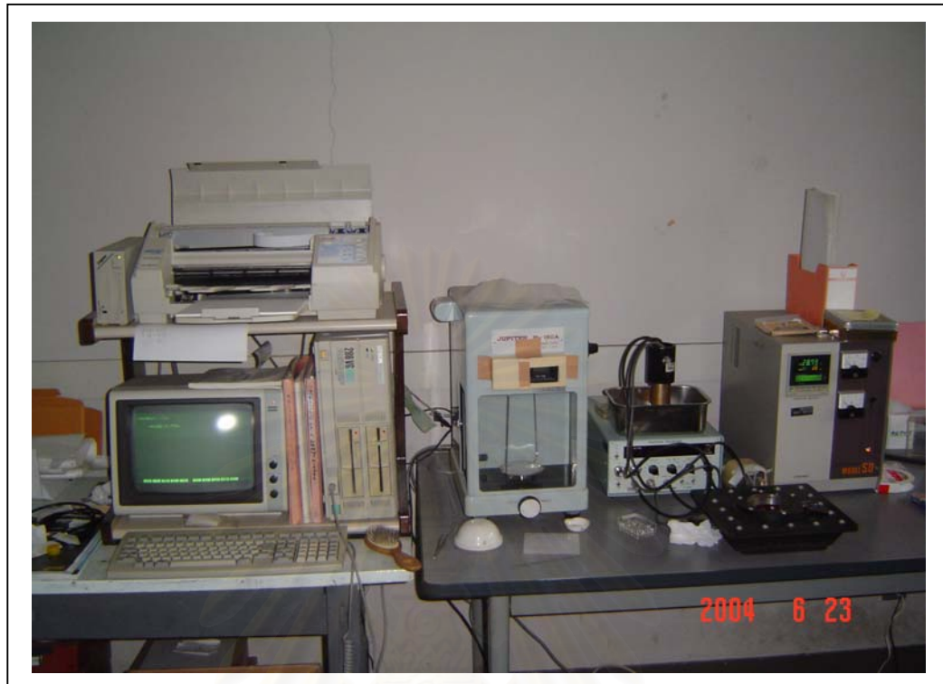
Figure 2.14 Kyokko 2500 TLD dosimeter at Akita University, Japan; that is used for TL glow curve measurement.
